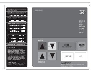
The indicator lights on the electronic console show you what information is being displayed. Information from five distinct fields as shown in Diagram 10 can appear: DISTANCE, TIME, SPEED, CALORIES, and INCLINE.
